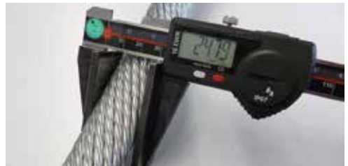
Fig. 4: Calliper with wide jaws
